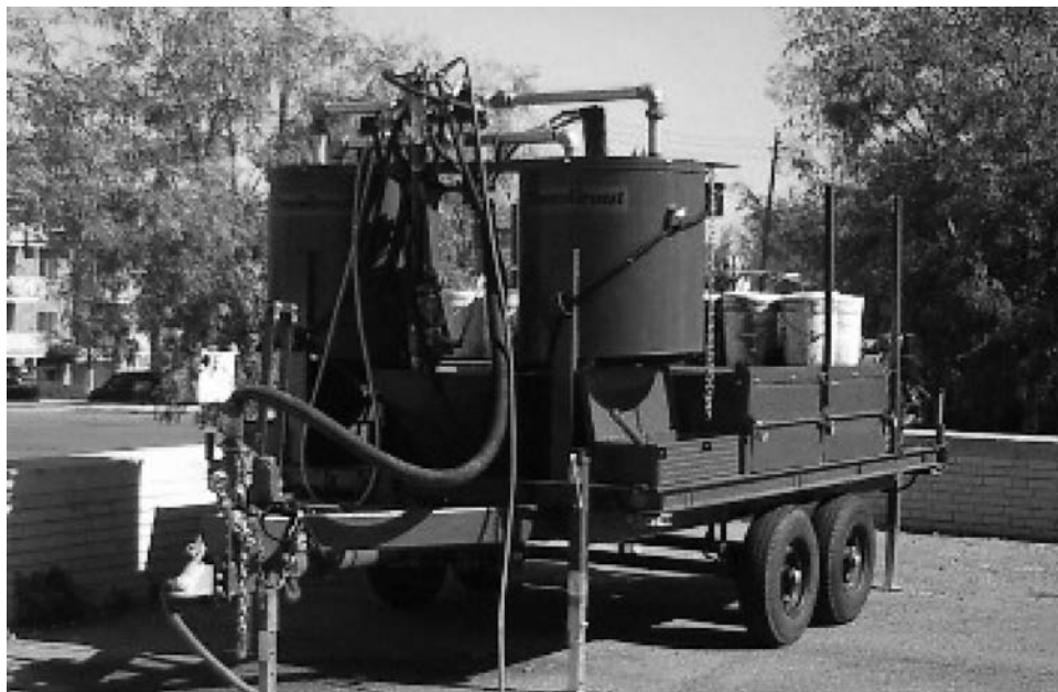
FIGURE 14.12 Hydrofracturing trailer setup, showing tanks for proppant and thickening agent (guar gum).
