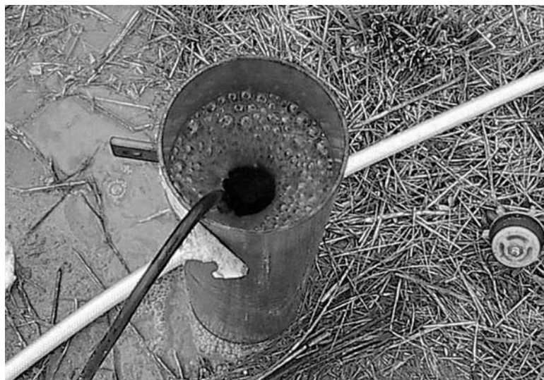
FIGURE 4.1 Oxygen bubbles erupting from the annular space between a monitoring well and its protective casing during a Fenton's Reagent application in a near-surface aquifer. Gases produced during these reactions can displace a significant fraction of the groundwater, reducing the hydraulic conductivity. Large gas eruptions can also generate safety hazards.
