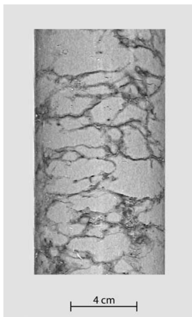
FIGURE 6.4 Reactive iron precipitation (dark areas) in a laboratory soil column. The column was packed by spooning P ne sand into a dry column, causing uneven compaction and the formation of strongly preferred pathways through the matrix. The injected reagent followed the more permeable pathways and precipitation quickly occluded them.
